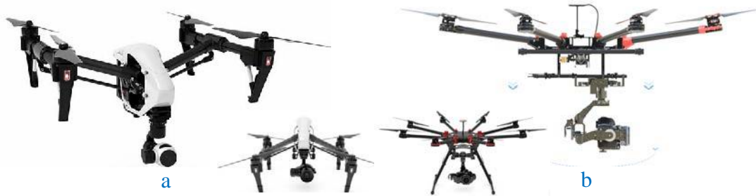
FIG.2 UAV type multi-copter with retractable landing gear, a.DJI Inspire 1 [1], b. DJI S1000 [4]
